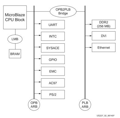
Figure 2: ML501 High-Level Block Diagram
